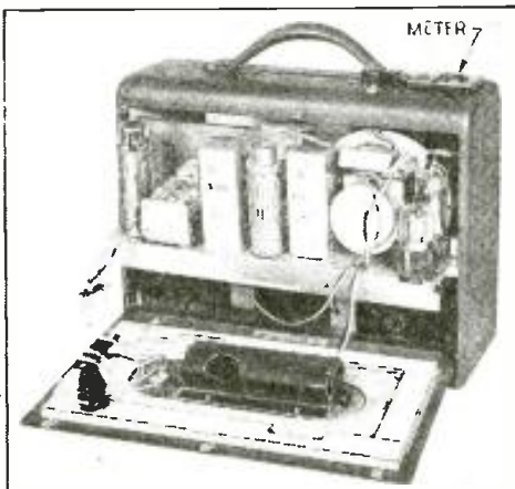
Exterior and interior views of the Sprague model IL-1 Interference Locator. The built-in loop antenna, mounted on back cover as shown in photo at right, may be supplemented by a rod antenna (see diagram, below).
